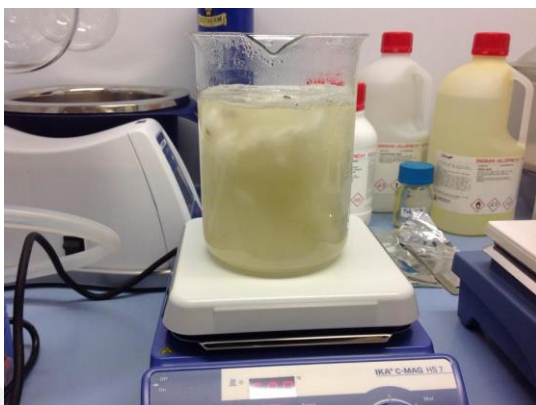
Figure 34. Silk cocoons boiling in hot water
