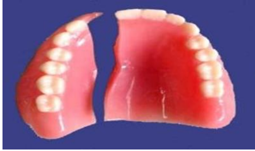
Figure 2.17: Images for Various Locations of Fracture for the Prosthetic Denture [88].
