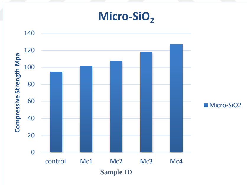
Figure 4.17: Compressive Strength Magnitudes For PMMA Samples After Adding Micro-Sio 2 in Various Ratios.
