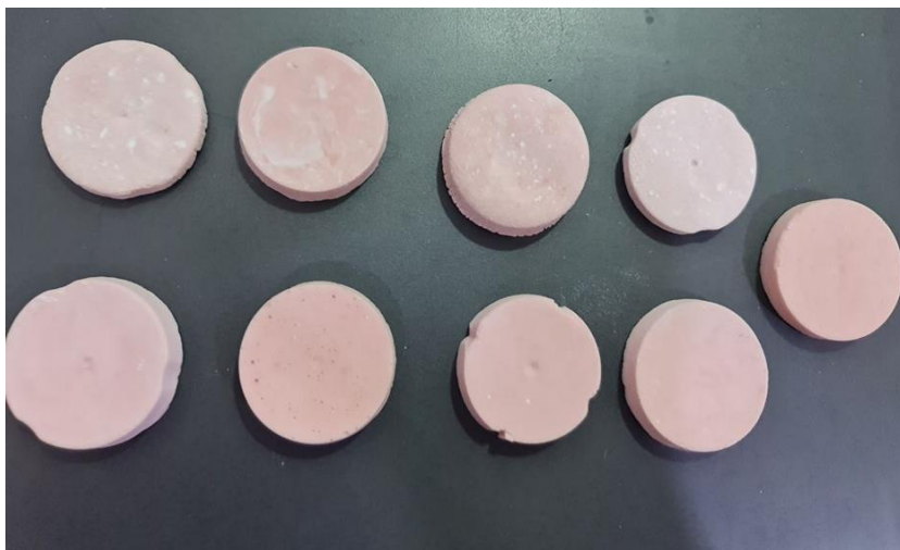
Figure 3.3: Casting Samples For Pure PMMA and PMMA Composite Strengthened By Micro and Nano ( \text{SiO}_2 ) Particles.
