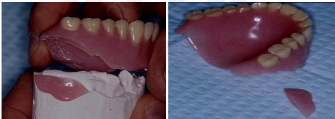
Figure 2.24: Images of Warpage Defect in the Prosthetic Denture [95].
