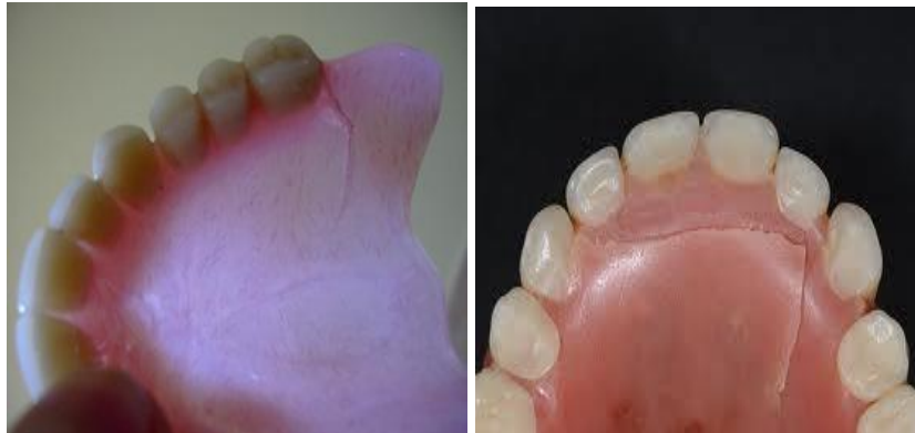
Figure 2.20: Images of Fatigue Fracture in the Prosthetic Denture [91].
