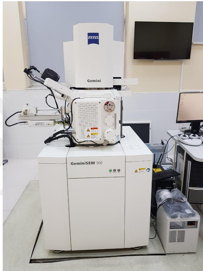
Figure 3.5. ZEISS GEMINI 500 SEM instrument.
