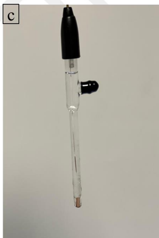
Fig 2. 2 a) Electrochemical set up with gamry featuring b) working electrode and c) reference electrode. (Karadas Research Group).
