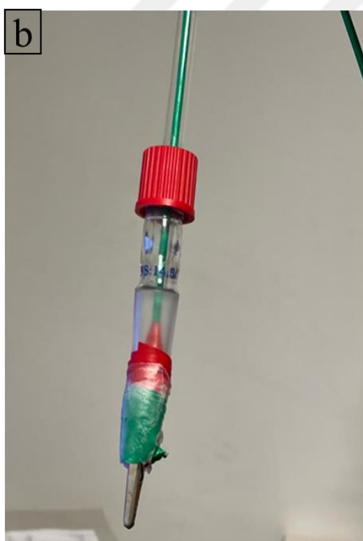
Fig 2. 2 a) Electrochemical set up with gamry featuring b) working electrode and c) reference electrode. (Karadas Research Group).
