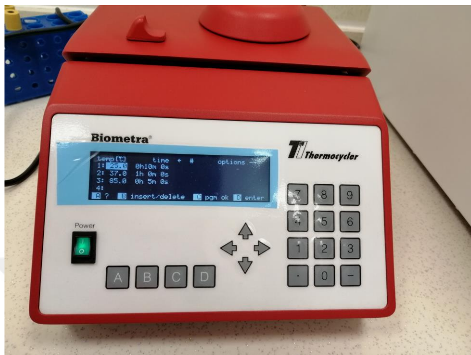
Figure 3.2: Thermocycler used for the reverse transcriptase reaction.
