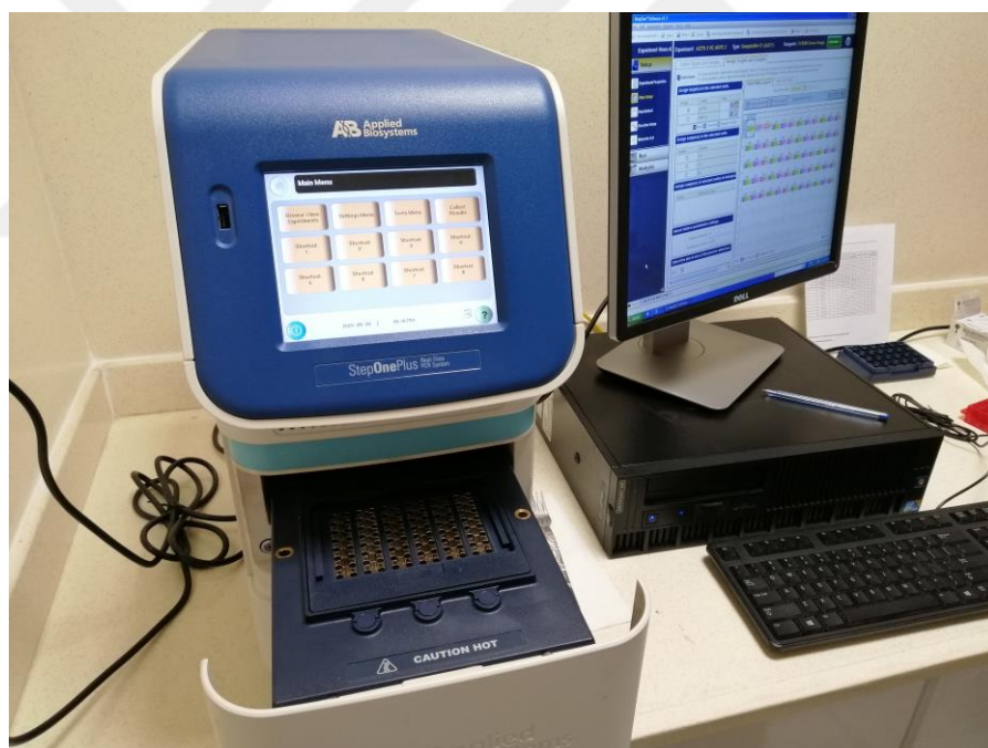
Figure 3.5: Real-time PCR device opened for the plate with the samples.
