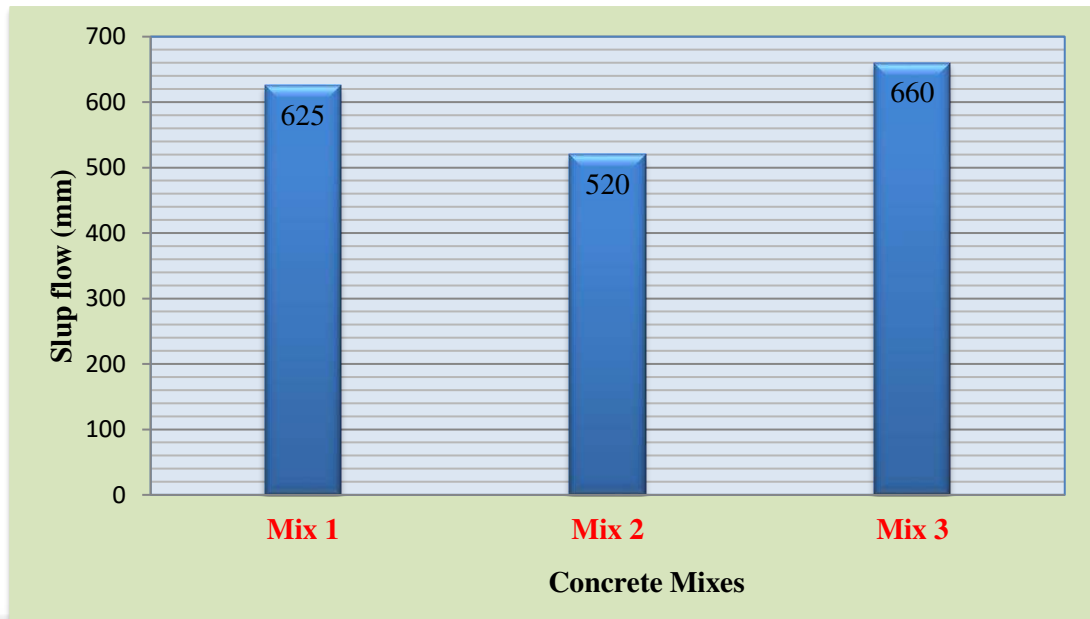
Fig 4.1 Variation of slump flow diameter and slump classes According to Efnarc (2005), SCC guide, SF1 class self-compacting concretes (625-650) can be applied to many normal structural members (e.g. walls, columns) T 50 slump flow times of the produced self-compacting concretes are presented in Fig 4.2. The T 500 slump flow time was generally less than 2.5 s except for the mixture (M2) remarkably increased the slump flow time of the SCC,
