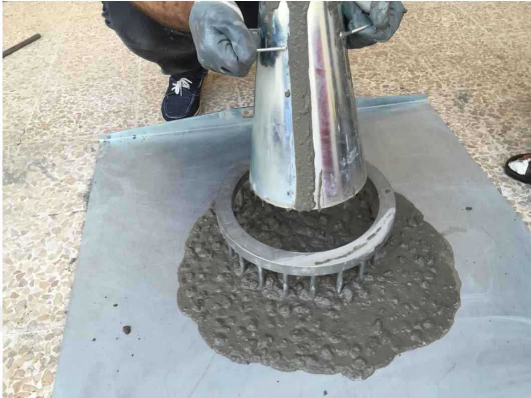
Fig (3.12) j-ring test
