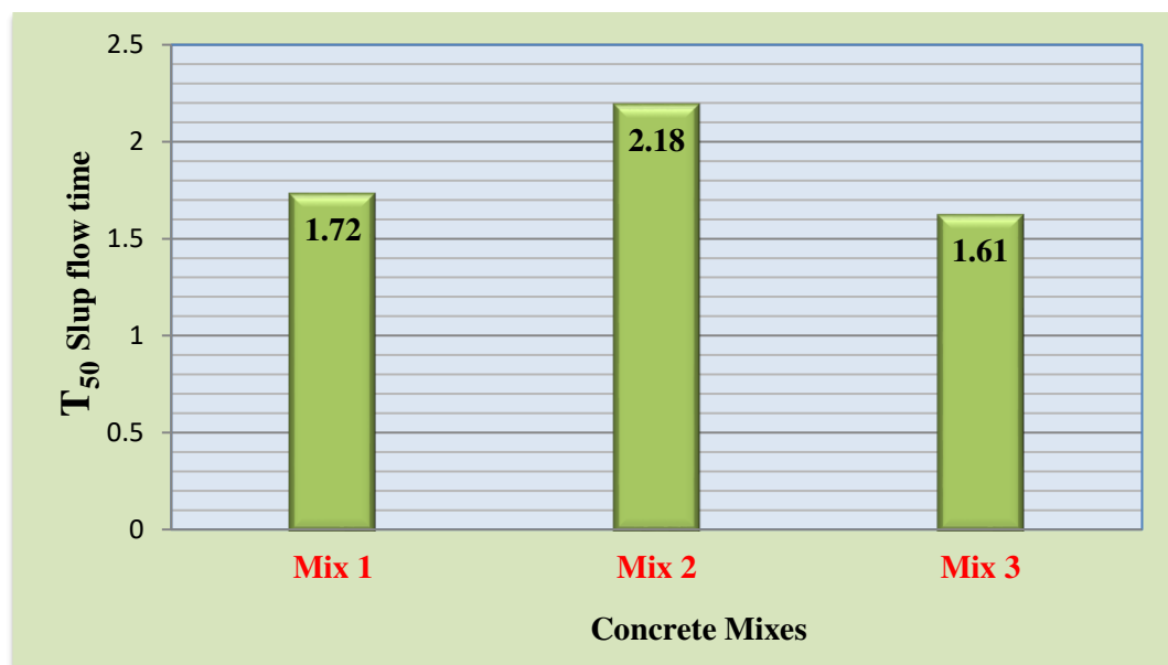
Fig 4.2 Variations of slump flow time and slump classes
