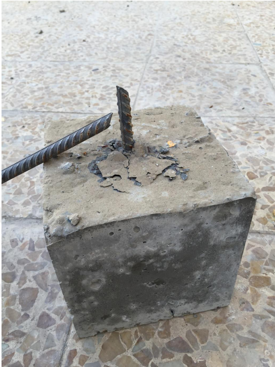
Fig (3.20) cut of the steel bar
