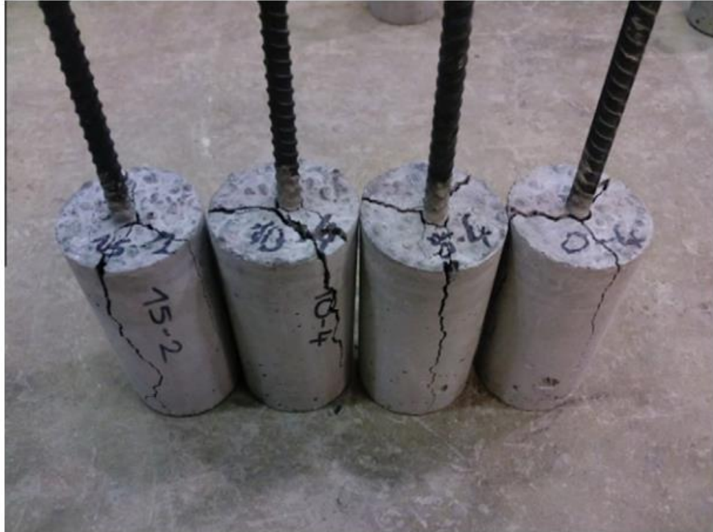
Fig 2.7 Typical crack pattern for SCLC specimens after pullout test (Karahane et al., 2012)
