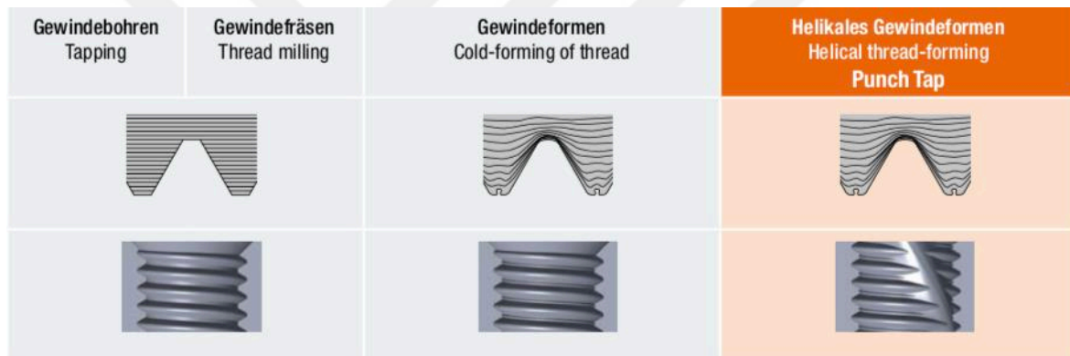
Figure 7 Comparison of Cut, Cold formed & Punch Tap Threads [12]
