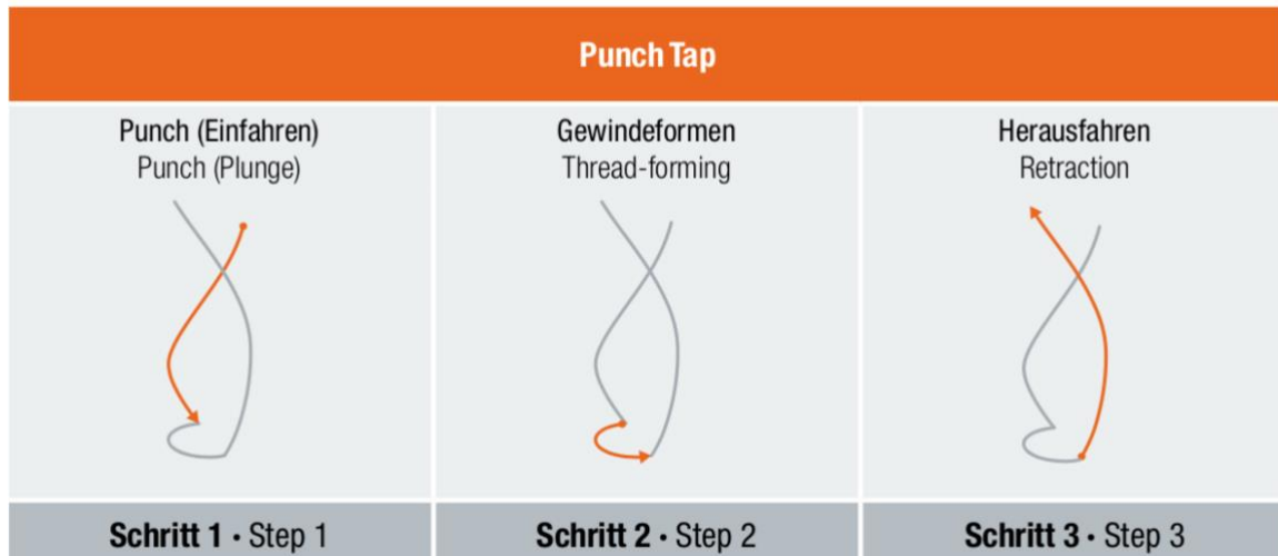
Figure 12 Working Mechanism of Punch Tap[13]
