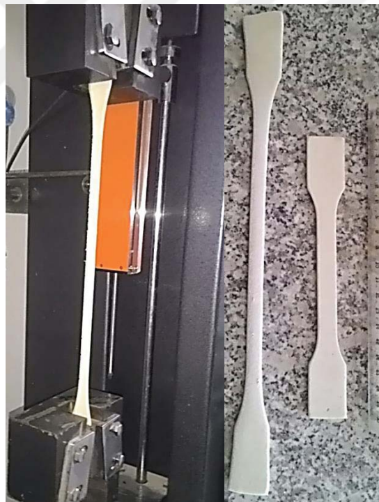
Figure 3.15 Elongation capability of 1-day cured TSL.
