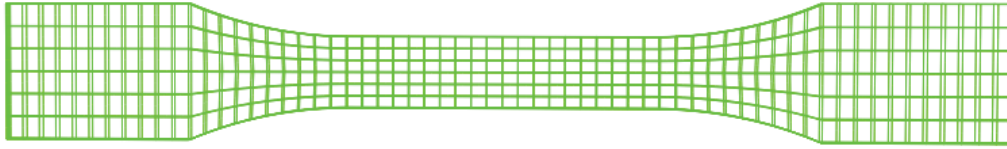
Figure 6.4 The mesh geometry of the specimen
