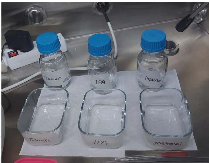
Figure 2.4: Chemical baths used for quenching.
