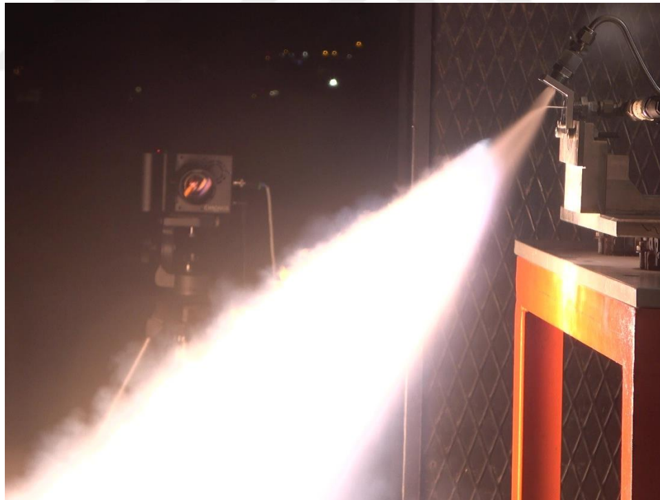
Figure 3.7: 60° ignition test with O/F ratio of 2.76.
