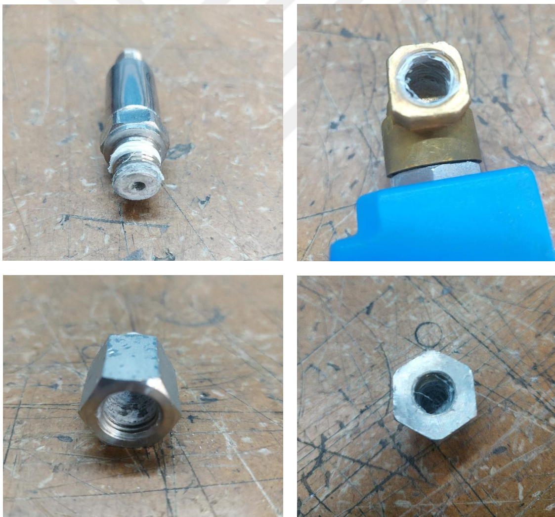
Figure 4.4: Post-test \text{Al}_2\text{O}_3 accumulation.
