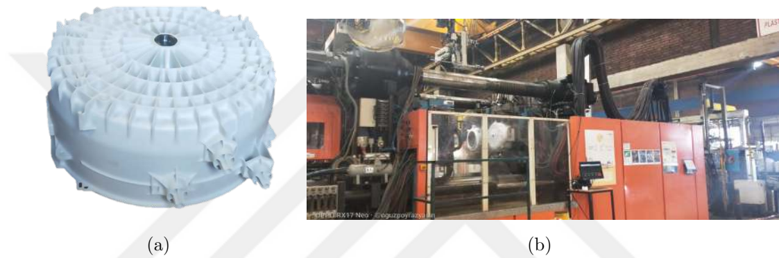
Figure 4.1: (a) The rear tub part of the washing machine, and (b) the 2000-ton Chen Hsong plastic injection machine.
