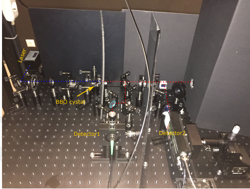
Figure 7.3: Experimental setup for noise to investigate the noise-embedded object detection.
