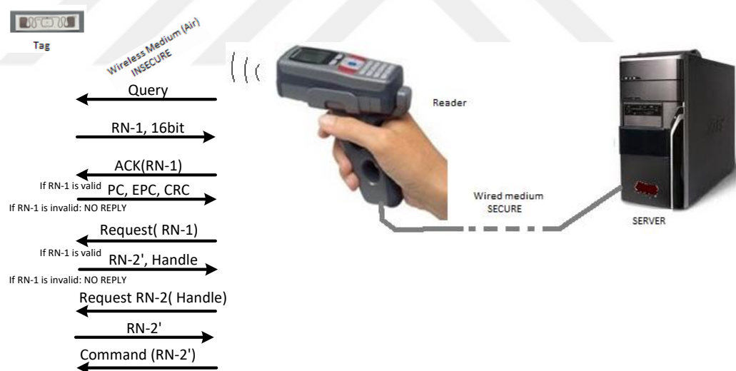
Figure 3.2 A typical UHF RFID tag reading scenario (Özcanhan, Dalkılıç & Utku, 2013)
