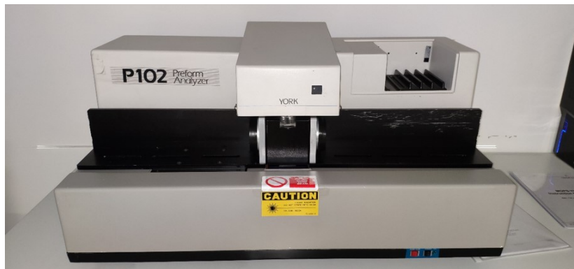
Figure 3.2: Preform analyzer is used to obtain RIP profile of the preform
