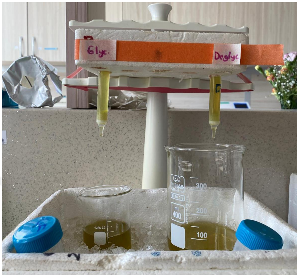
Figure 3.7. Affinity chromatography system for purification of FLAG tagged proteins
