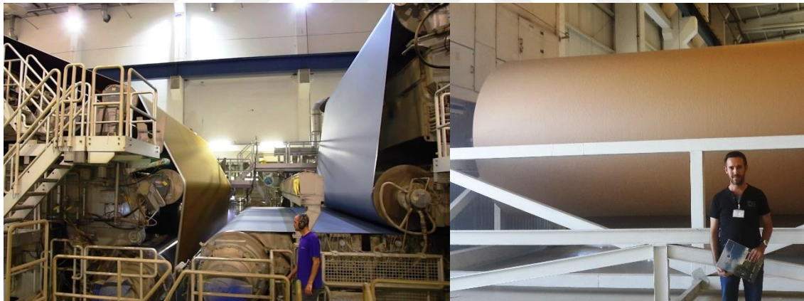
Figure 4. Giant screens to dry the refined paper pulp and rolls of paper.
