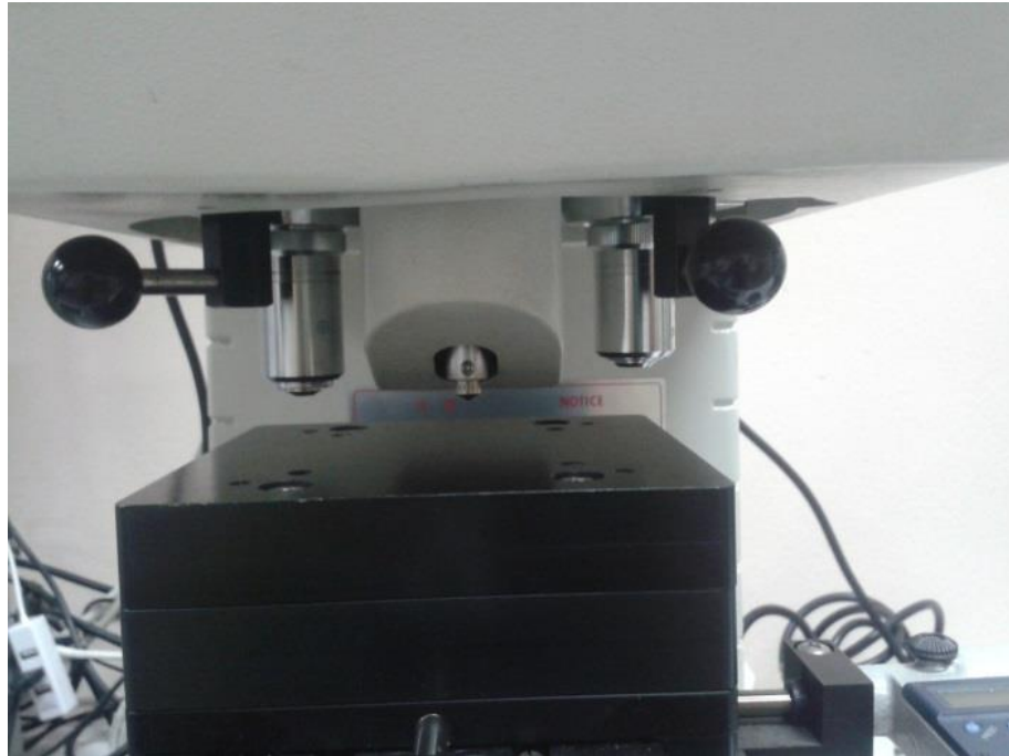
Figure 2.3.7 The Vickers indenter of HMV Shimadzu microhardness tester
