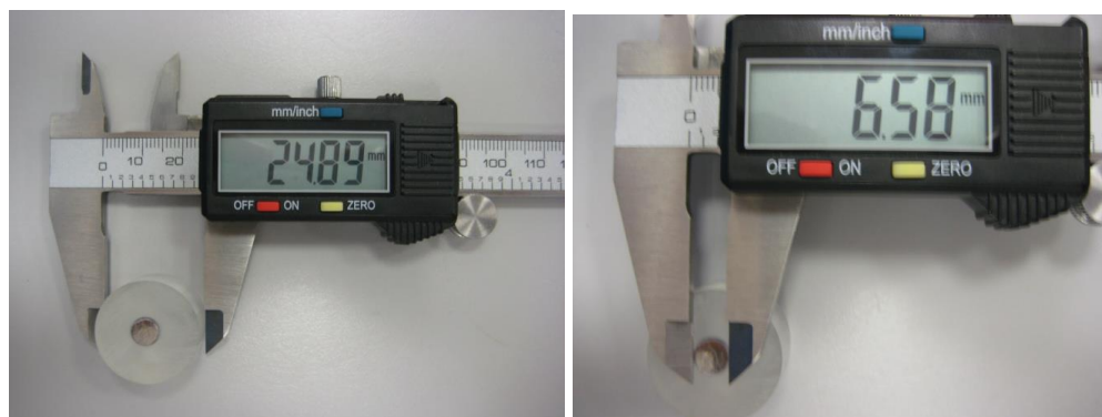
Figure 3.1.3 Polished sample with the radius of 6.58 mm
