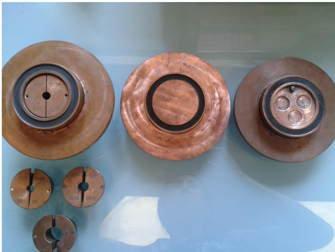
Figure 2.2.2 Different types of copper hearts depending on the usage
