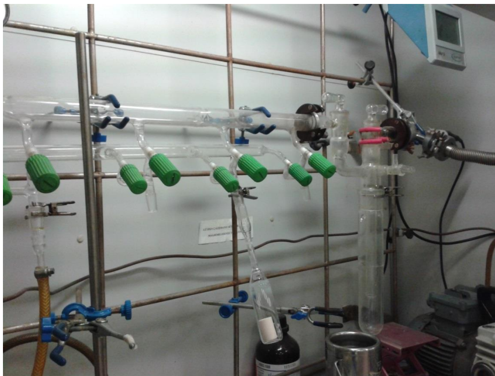
Figure 4.1.5 The silica reaction vessel connected to the vacuum line
