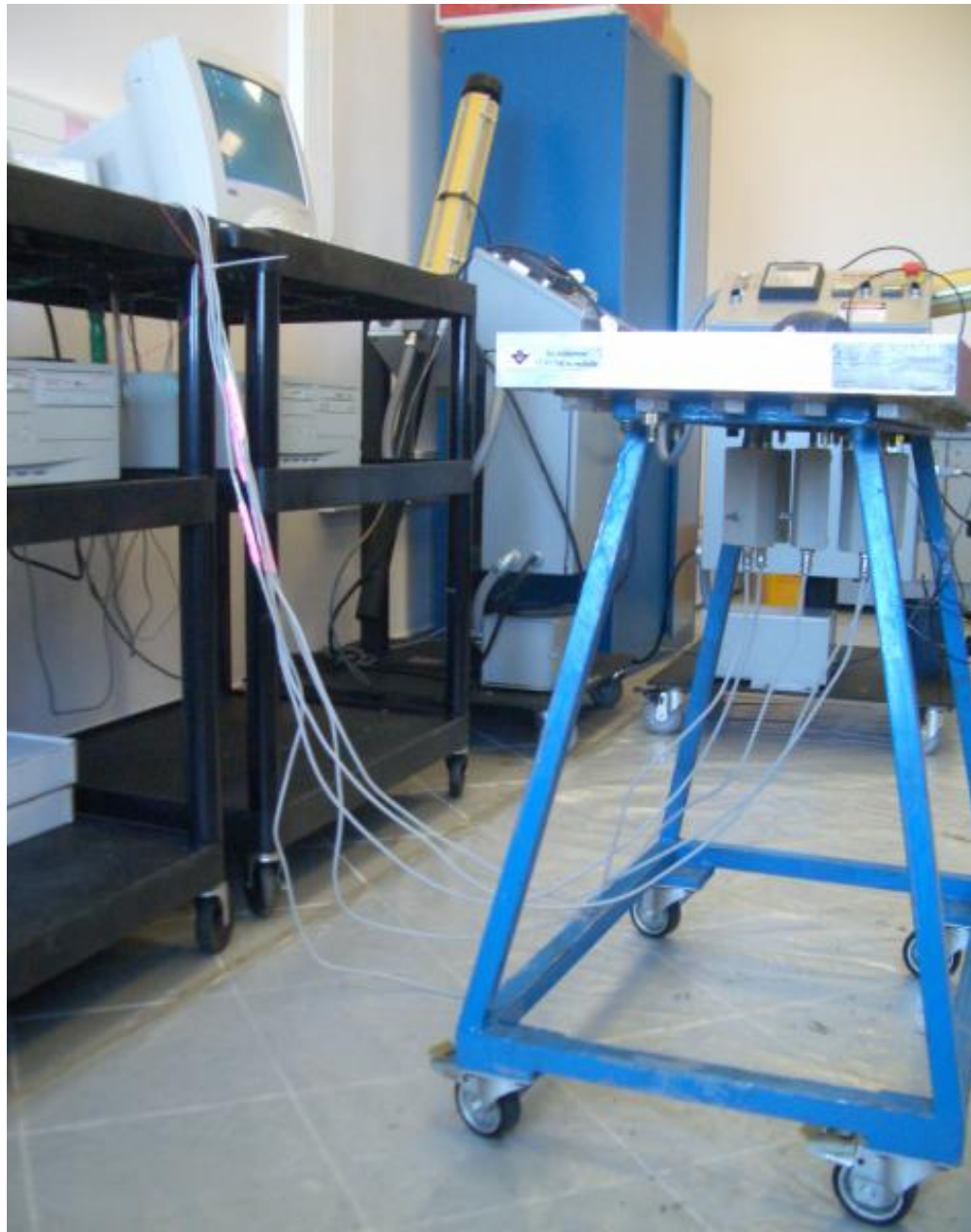
Figure 5.23 Another picture of point voltage sensors mounted on the mold, and the cables of the sensors are connected to the DAQ and power supply.
