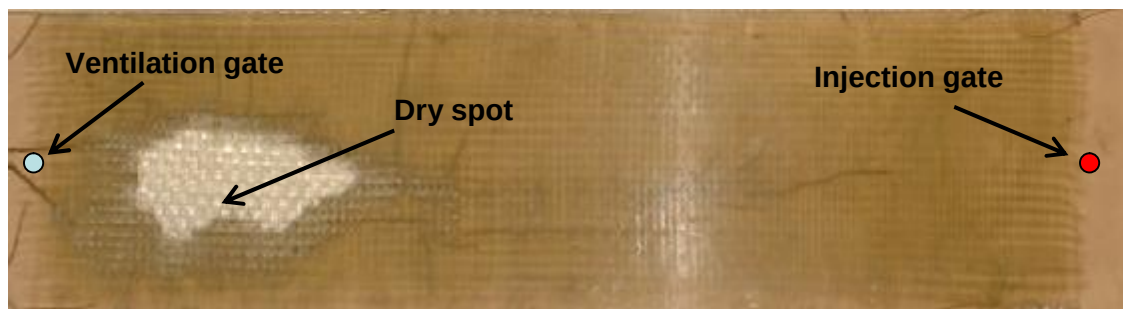
Figure 3.7 A composite part with a macro size dry spot (void) near the ventilation gate.
