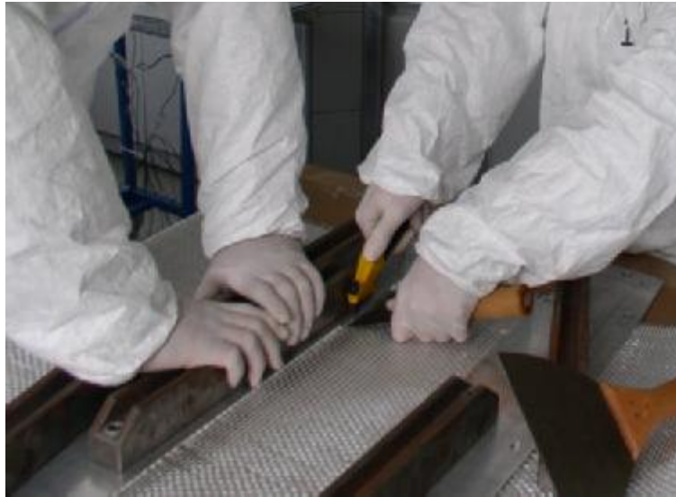
Figure 3.2 Manual preform preparation.
