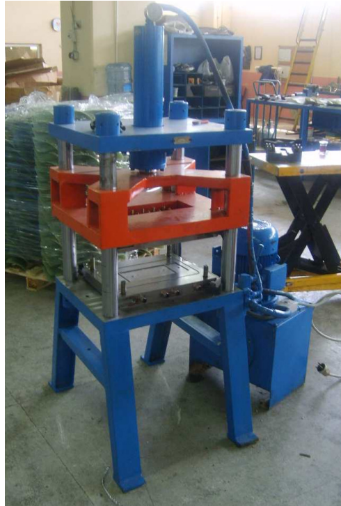
Figure 4.22 Hydraulic press with the mold.
