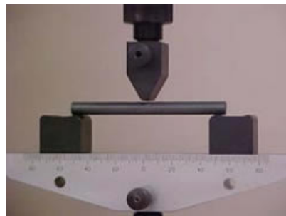
Figure 6.1 Three-point bending test [35].
