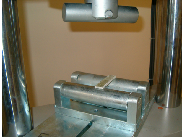
Figure 6.3 The three-point bending apparatus in our university.
