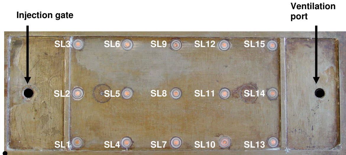
Figure 3.8 Sensor configuration on the lower mold cavity.
