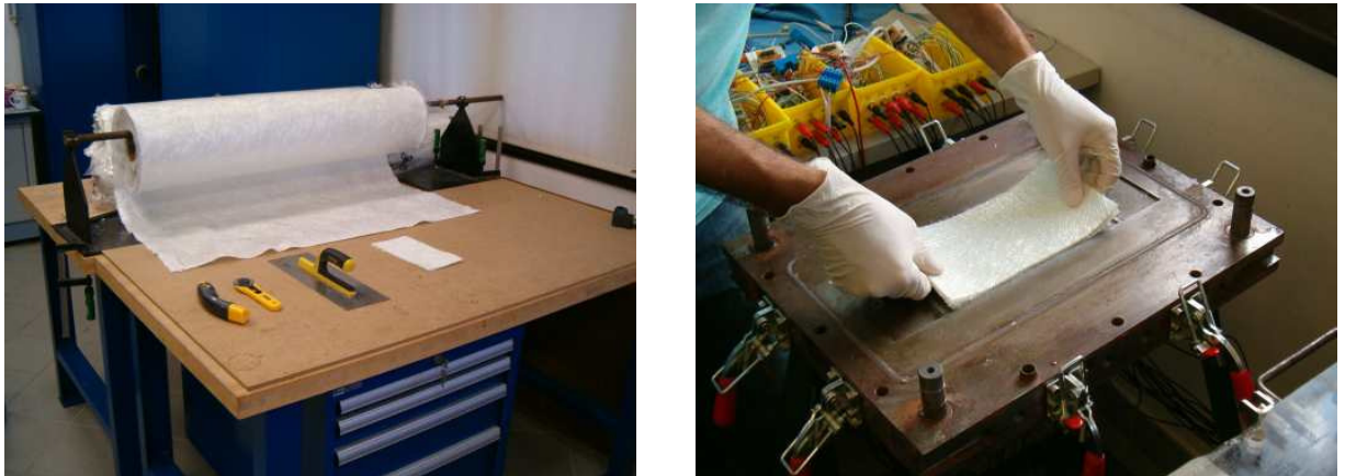
Figure 4.24 Fabric roll and placement of fabric preform into the mold cavity.
