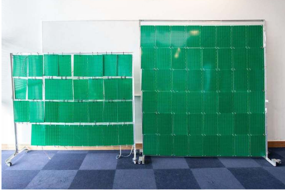
Figure 1.5: Rfocus: Real implementation of an RIS [8].
