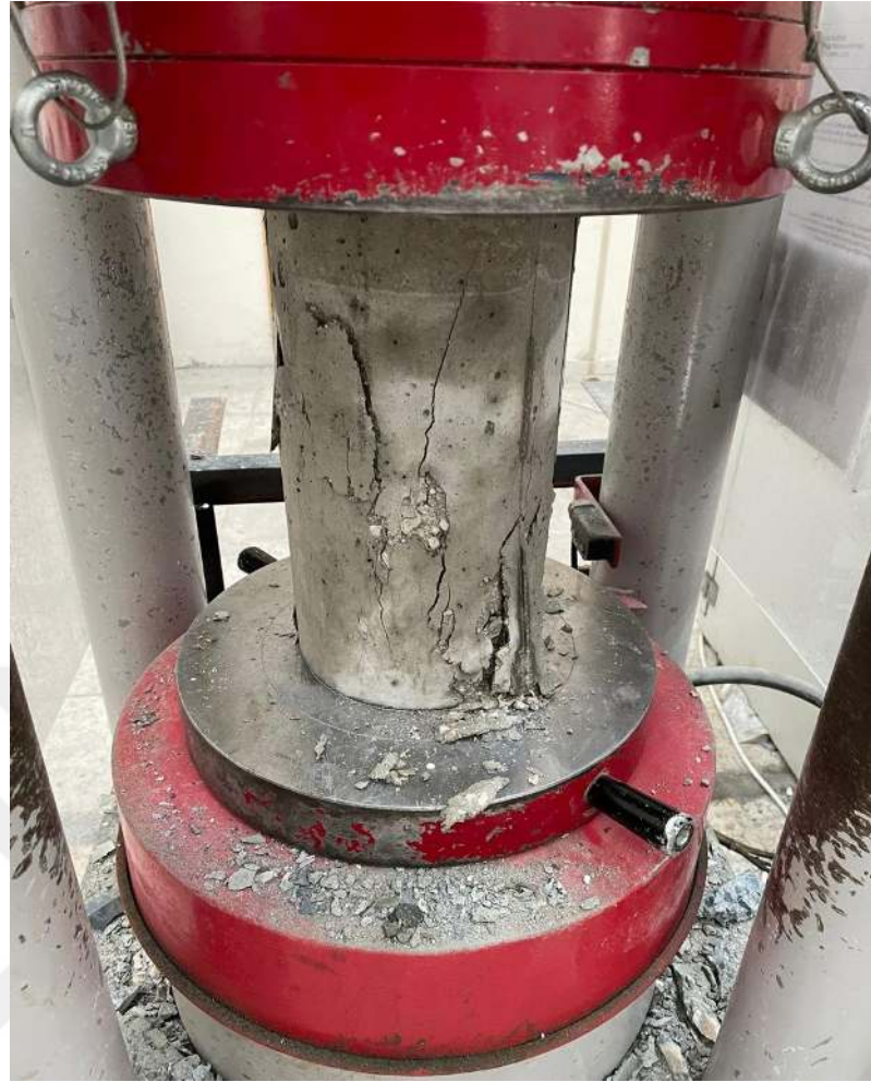
Figure 3.4: Cylinder Pressure Test
