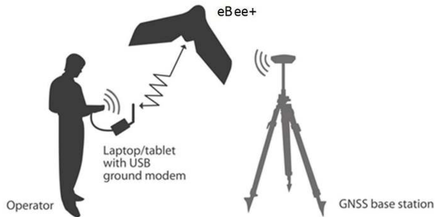
Figure 3.4. UAV Data acquisition with GNSS base station ( http-4 )
