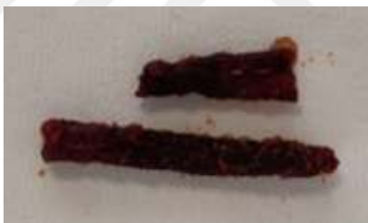
Figure 4.3: Polymerized samples of bulk polymerization. Samples were fully polymerized.
