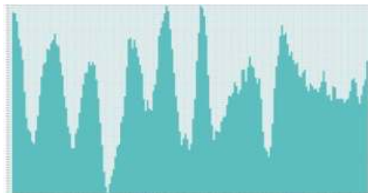
Figure 4.16: 1D projection of the red rectangle area in Figure 4.16. Distance between the first and eighth peak is 1.75 nm.
