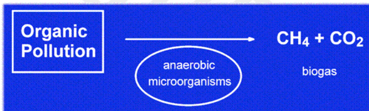
Figure 2.4. Conversion of organic pollutants to biogas by anaerobic microorganisms [66].
