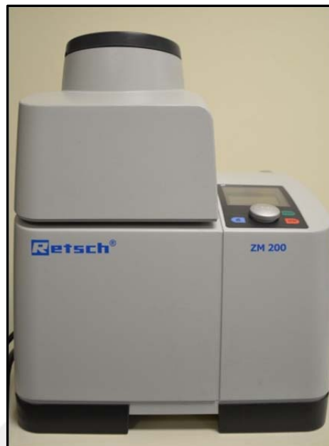
Figure 17. Centrifugal grinder used for grinding the adsorbent materials
