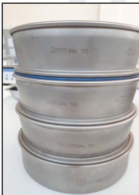
Figure 18. Retch brand sieves (left) and sieve shaker (right) used to screen the ground adsorbent materials
