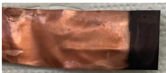
Figure 3. 4 Image of the cathode surface after the experiment performed at 8 V for 1 hour
