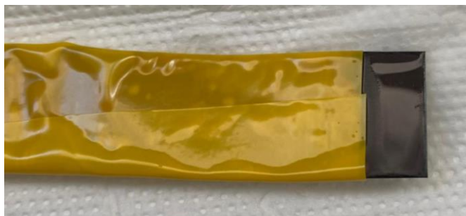
Figure 3. 7 Image of copper foil cathode after the experiment performed 13 V, 1 hour, 2cm2 conditions
