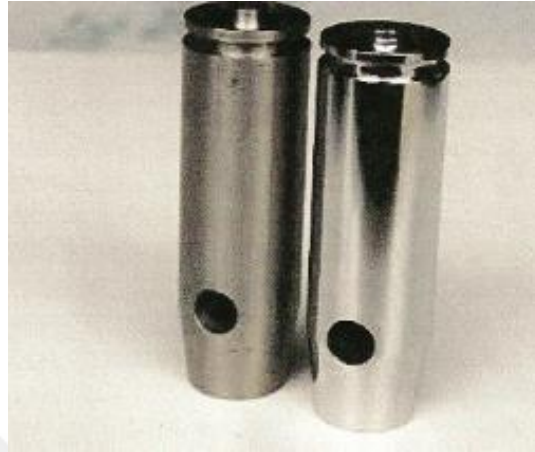
Figure 1. 2 Images of the non-electropolished and electropolished samples [15]
