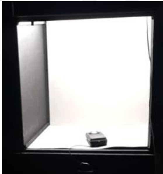
Figure 26. NCS Colour meter (left) and Konica Minolta Illuminance Meter T-10A in the experiment box (right) (personal archive of Begüm Ulusoy).
