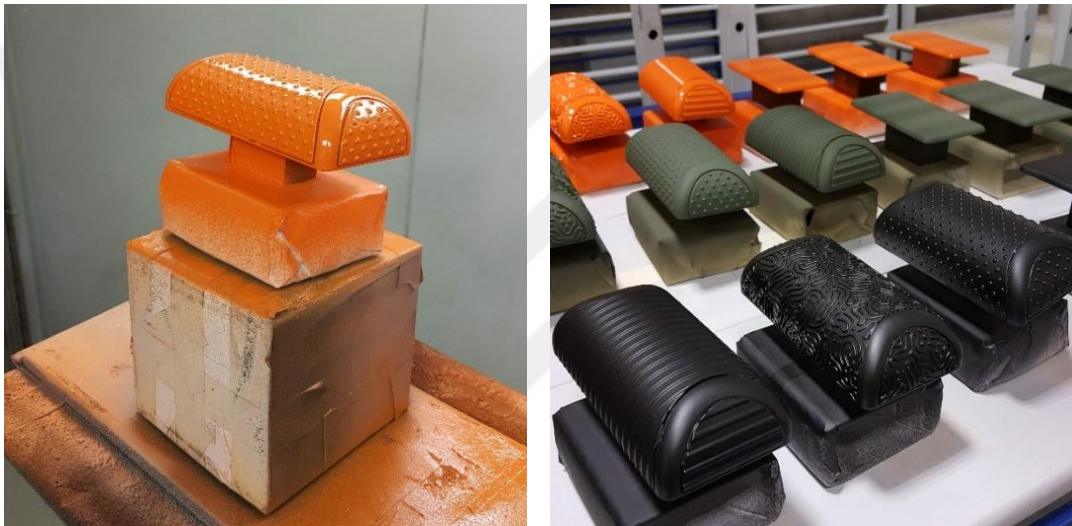
Figure 4.9. Coating process; black, green and orange
