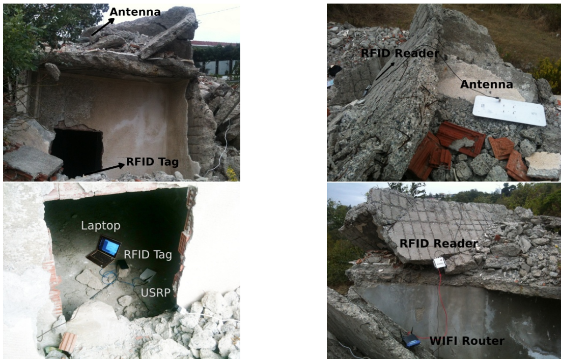
Figure 6.4: Images of experiment setup in the area with ruins.
