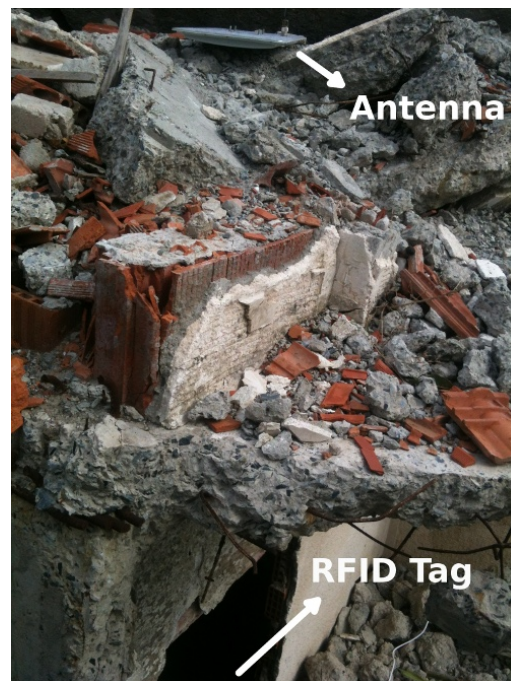
Figure 6.5: Medium between antenna and passive RFID tag.
