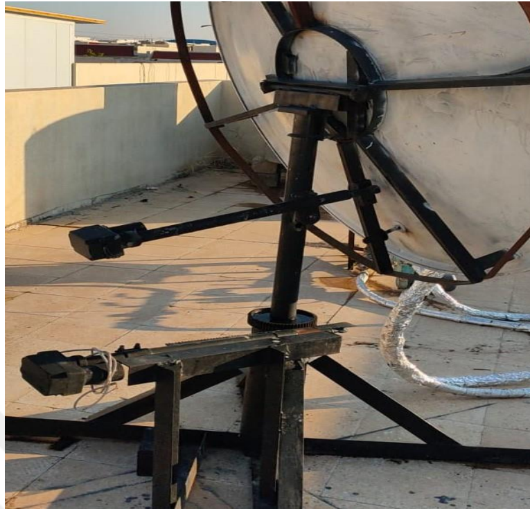
Figure 3.5 Solar dish base
