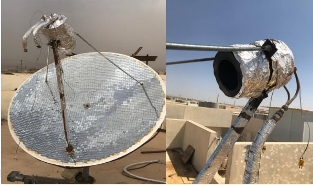
Figure 3.4 Receiver setup on the dish
