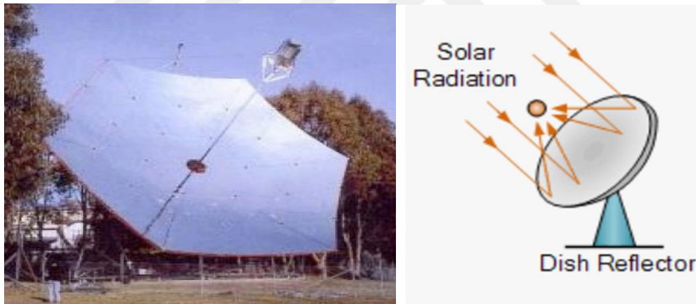
Figure 1.6 The Parabolic Dish Collector (Abbott 2009)
