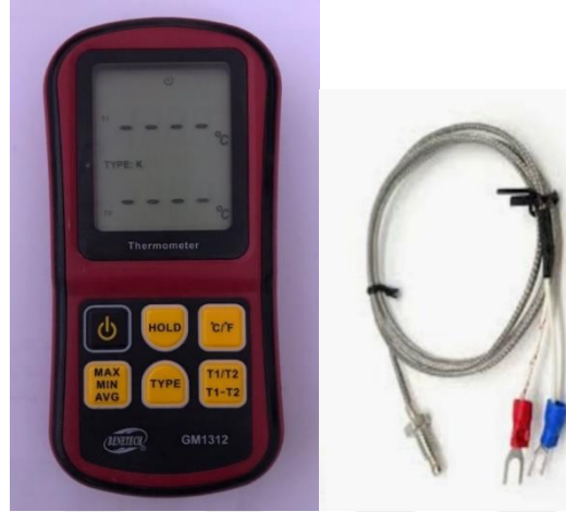
Figure 3.10 Temperature measuring devise (left) along with the thermal sensors k-type (right)
