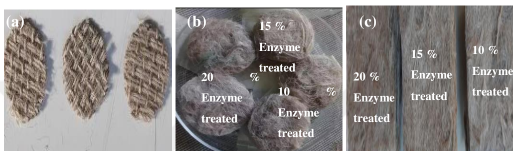
Figure 3.17. Samples for test: a) Neat enset fabric. Cellulosic enset nanofiber: b) Sound absorption c) Air permeability
