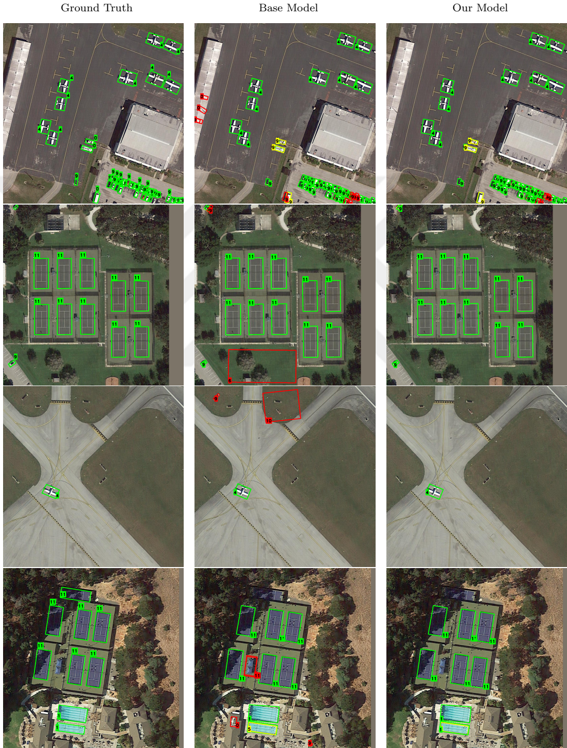
Figure 5.11: Effect of class probability threshold on DOTA detection results. Each row represents a scene. Colors: green (correct), yellow (wrong class), red (false positives). Columns (left to right): ground truth, oriented R-CNN baseline (threshold 0.01), proposed model (threshold 0.01). The proposed model achieves similar recall but improved precision over the baseline.
