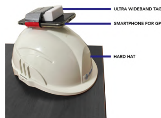
Figure 3.5. UWB tag and IOS smartphone implementation to hardhat.
