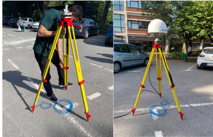
Figure 4.2. Referential point PB antenna settlement.
