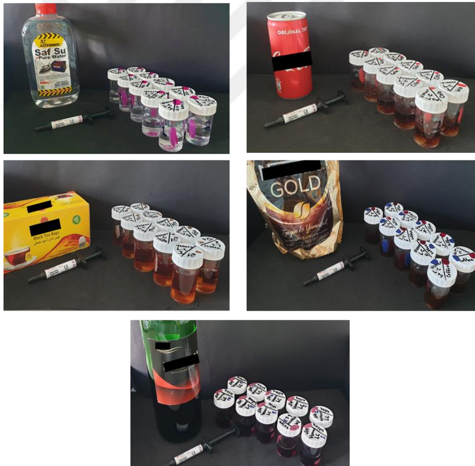
Figure 32. Grouping of 3M Rely-X Veneer Light-Cure (3M.LC) specimens according to the solutions (distilled water, cola, tea, coffee, and red wine)
