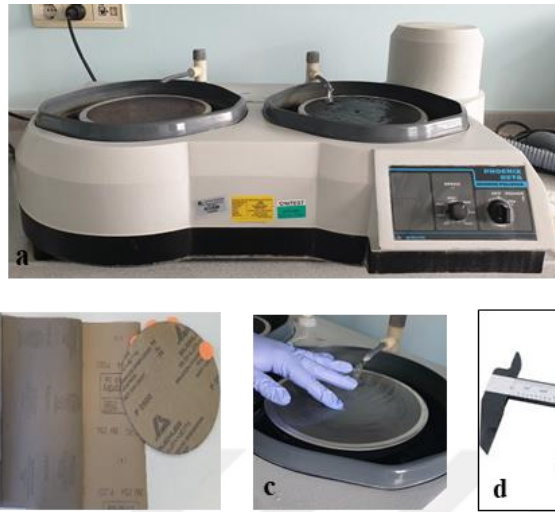
Figure 28- a. Grinding and polishing machine, b. SiC grinding sheets, c. Grinding and polishing procedure, d. Digital caliper.
