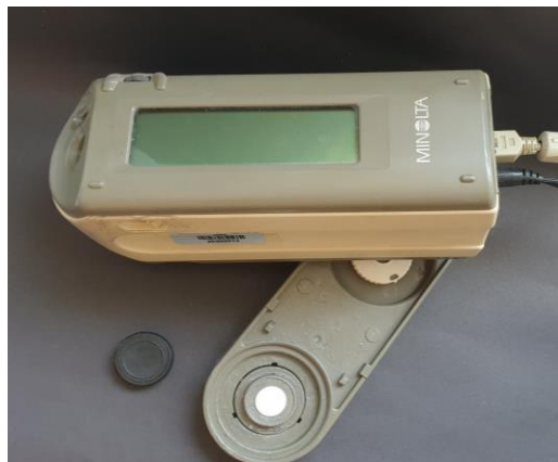
Figure 36. Spectrophotometer device (CM-2600d, Konica Minolta Sensing Inc., Japan).
