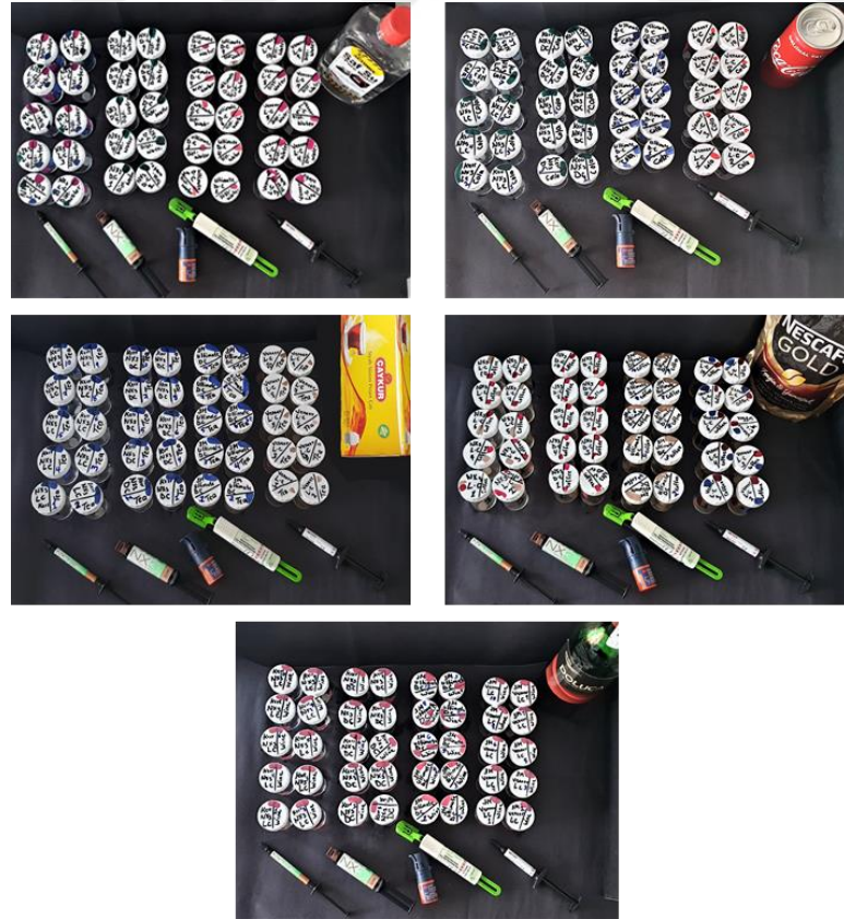
Figure 31. Grouping of all of the specimens and their vials used for immersion.
