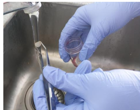
Figure 30. Washing the specimens under running water.
