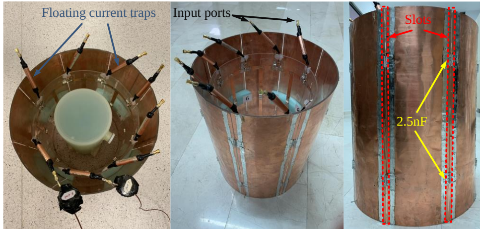
FIGURE 3.2 – The manufactured structure of a shielded 8-channel degenerate birdcage TxArray coil loaded with a cylindrical sodium-nickel solution phantom. The shield is broken down into eight uniformly spaced segments, where the adjacent segments are connected via two 2.5 nF capacitors at positions facing the coil's end-rings. Eight floating current traps were constructed and added to the coil.
