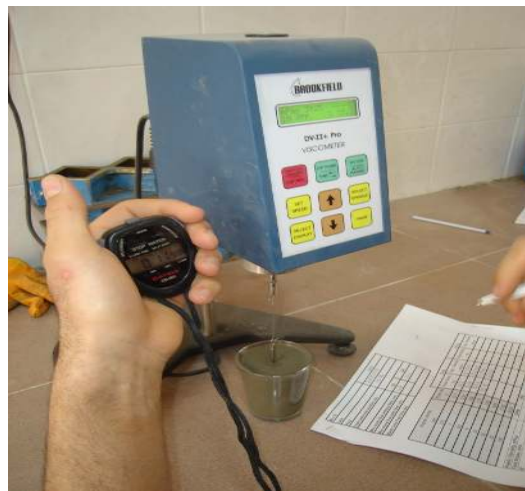
Figure 3.8 Rotational viscometer test
