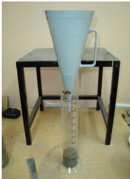
Figure 3.7 Marsh cone test
