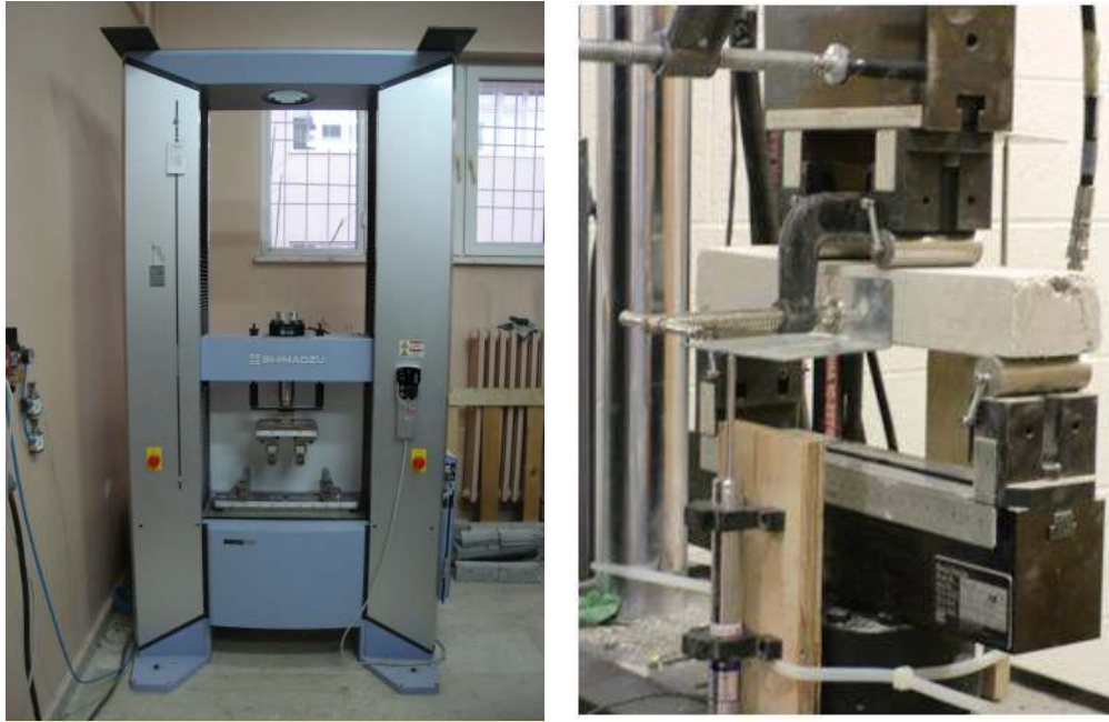
Figure 3.11. Four-point Flexural Strength test machines
