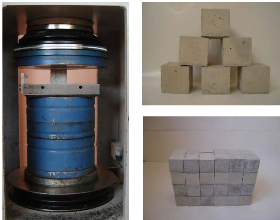
Figure 3.9 Compression testing machine and cubic samples
