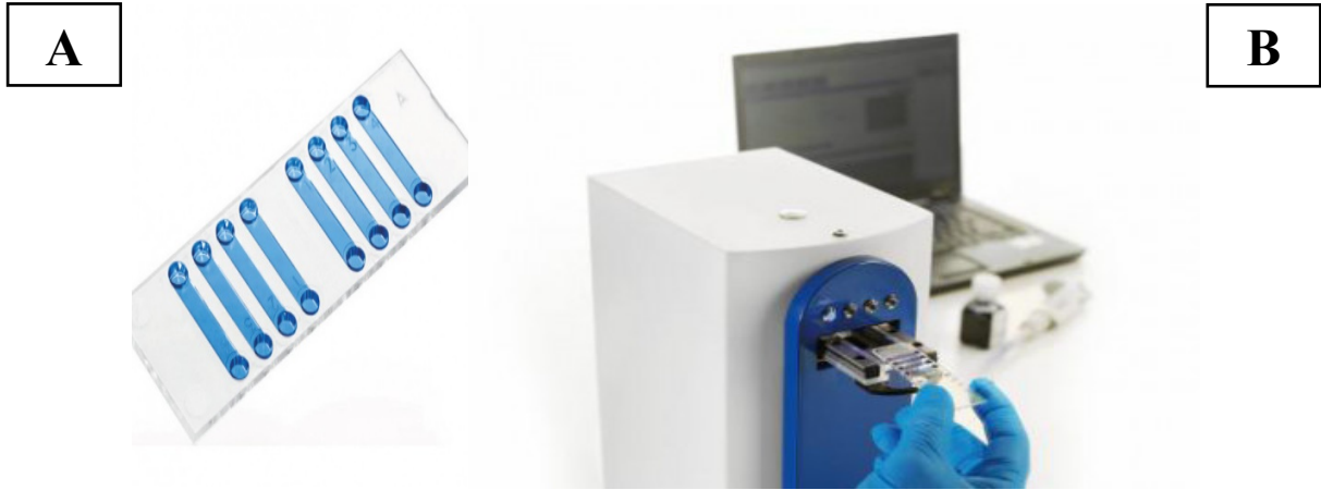
Şekil 4.2. Cedex smart slide (A) ve Cedex XS otomatik hücre sayıcı (B) ( http-12 )
