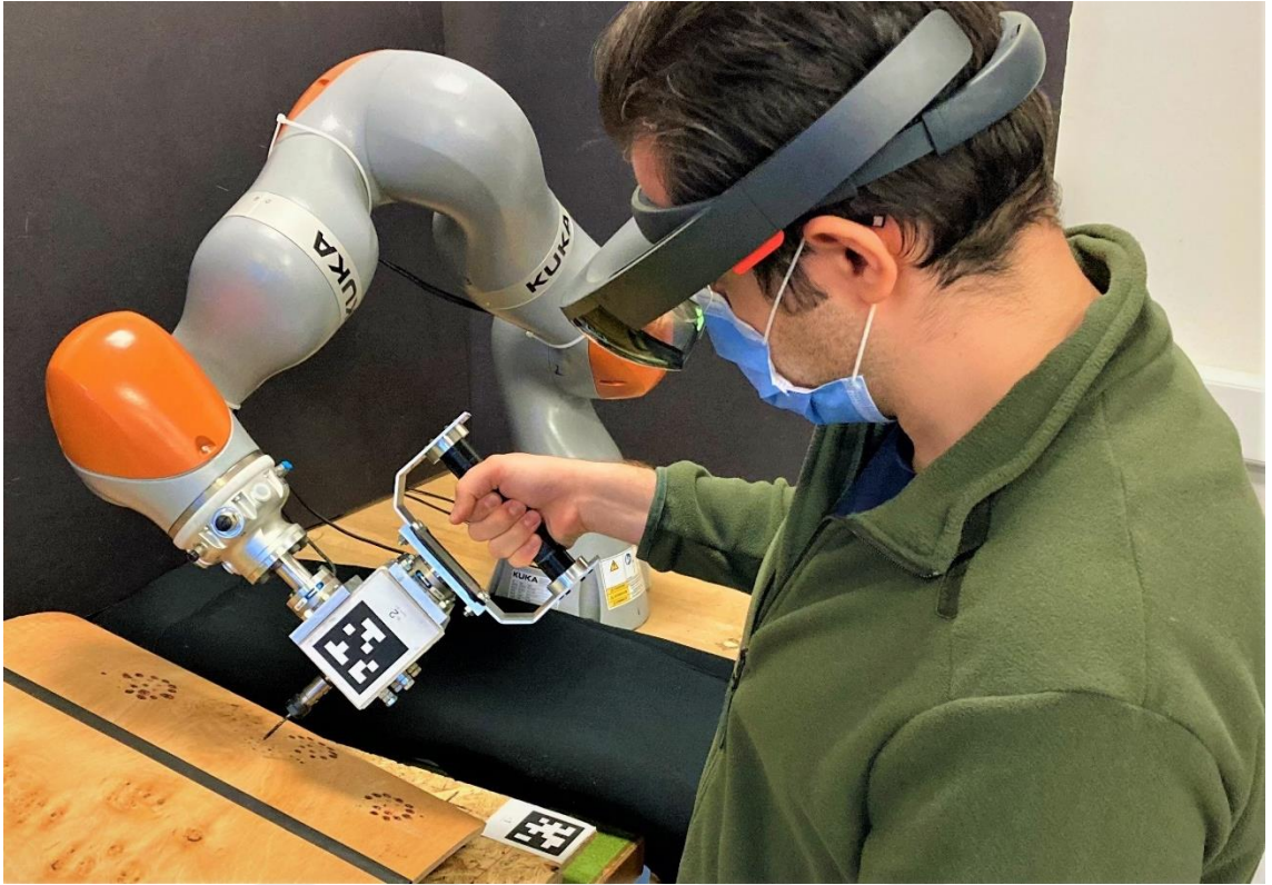
Figure 1, Our pHRI system designed for drilling on a curved surface consists of a cobot, a drill attached to it, two force sensors, and a HoloLens AR goggle.
