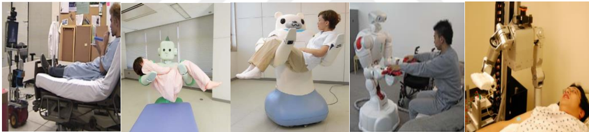
Figure 2.9. Left to right: (1) Clara assisting with spirometry exercise (Kang et al., 2005); (2) Human care task with RI-MAN (Onishi et al., 2007); (3) RIBA lifting a subject (Mukai et al., 2010); (4) TWENDY-ONE aiding in breakfast preparation (Iwata and Sugano, 2009); (5) Cody positioned by the patient bed (King et al., 2010).
