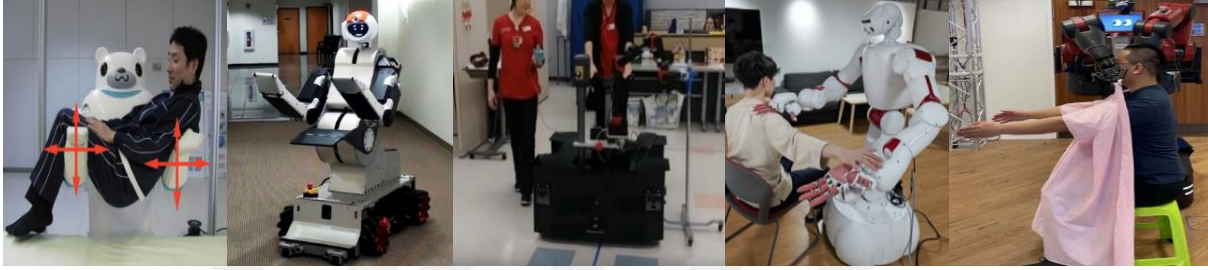
Figure 2.10. left to right: (1) Lifting experiment with RIBA (Ding et al., 2012); (2) RoNA prototype for patient lifting (Ding et al., 2014); (3) DOLA assisting subjects (Abubakar et al., 2020); (4) Physical exercises with Dry-AIREC (Miyake et al., 2022); (5) Robot dressing patient (Zhang and Demiris, 2023).
