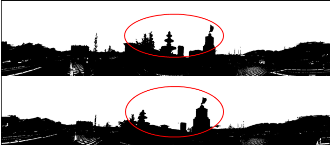
Figure 2.1. Change of Skyline as Real Location of Robot Changes
