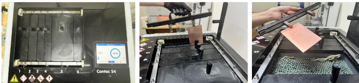
Figure 8.47. Stages of hole plating
