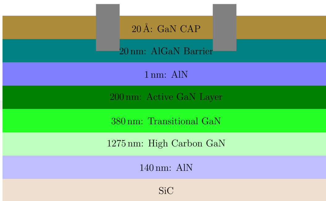
Figure 2.9: Illustration of Layers After Ohmic Contacts
