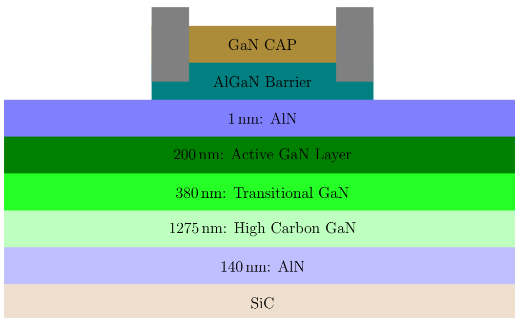
Figure 2.10: Illustration of Layers After Mesa Etch
