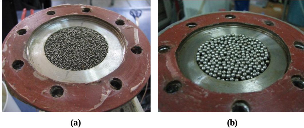
Figure 3.2 : Packed beds of (a) 1-mm steel spheres, (b) 3-mm steel spheres.
