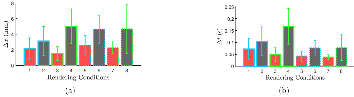
Figure 4.4: Thresholds to discriminate two consecutive virtual edges in EXP-1 (mean values and standard deviations); a) spatial threshold, and b) temporal threshold. Red and gray bars are for FF \rightarrow RF and RF \rightarrow FF , solid and dotted bars are for f_v of 30 and 60 mm/s, blue and green bars are for V_{amp} of 1 and 2 \mu\text{m} , respectively.
