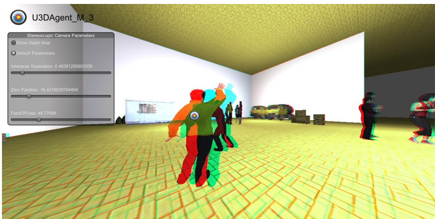
(c) Stereo camera parameter adjustment menu shown upon locking onto a scene-element.
