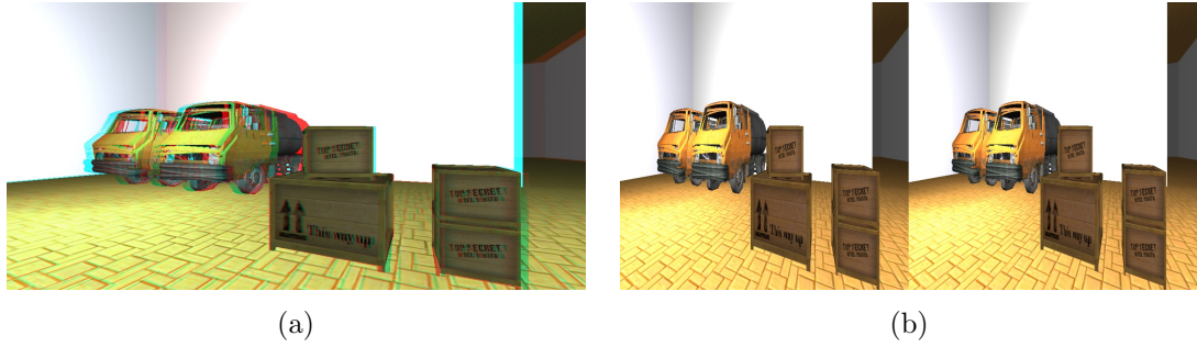
Figure 10.4: Available stereo-output settings of the framework (a) red-cyan anaglyph output (b) side-by-side output (before being overlapped by the display device).
