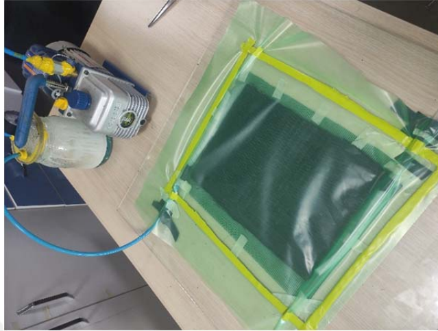
Figure 3.7. Composite plate production by vacuum infusion method
