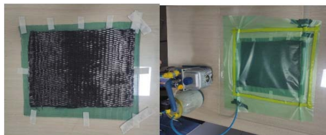
Figure 3.6. Composite plate production by vacuum infusion method
