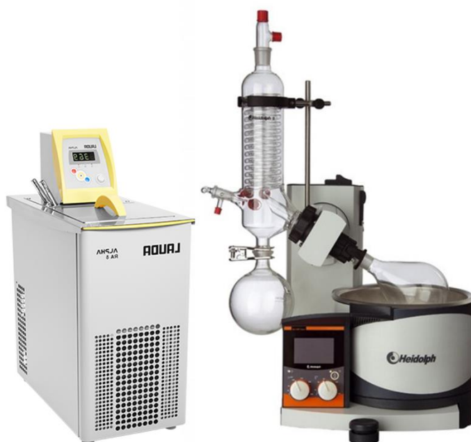
Figure 3.2. Lauda Alpha RA 8 with a Heidolph Rotatory evaporator to remove the solvent from extracts.
