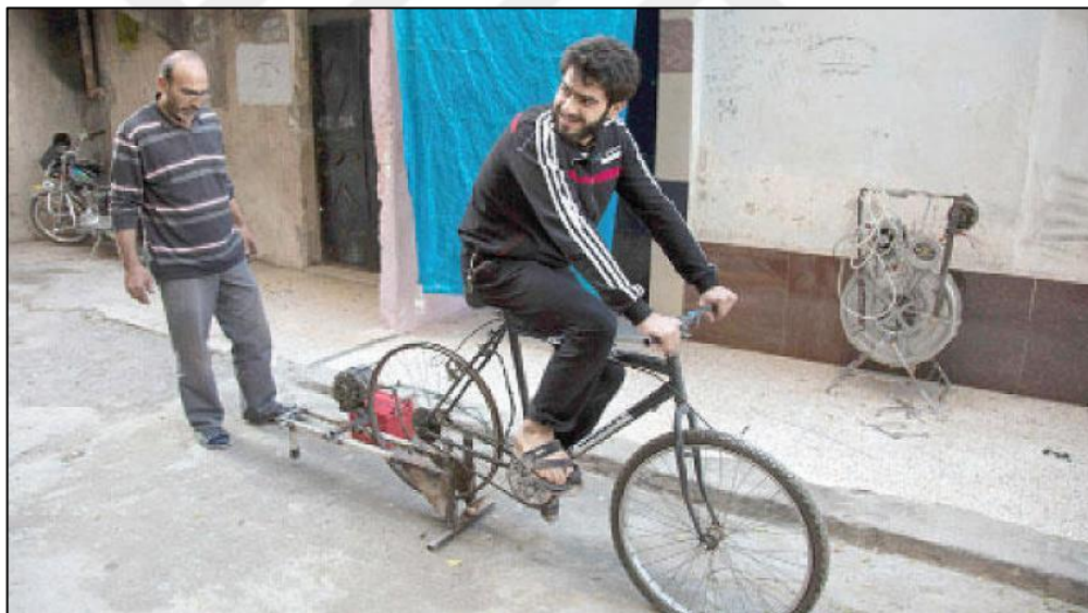
Figure 5.8. Bicycle power generator in Aleppo, 2016 [63].
