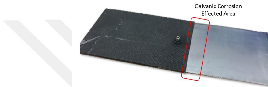
Figure 4.6. The region where the galvanic corrosion effect was examined on the aluminum AA2024-T3.
