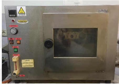
Figure 3.2 Rolling Thin Film Oven Test (RTFOT) device (Personal archive, 2019)
