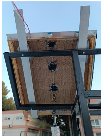
Figure 7.28. Test setup of the cooled panel
