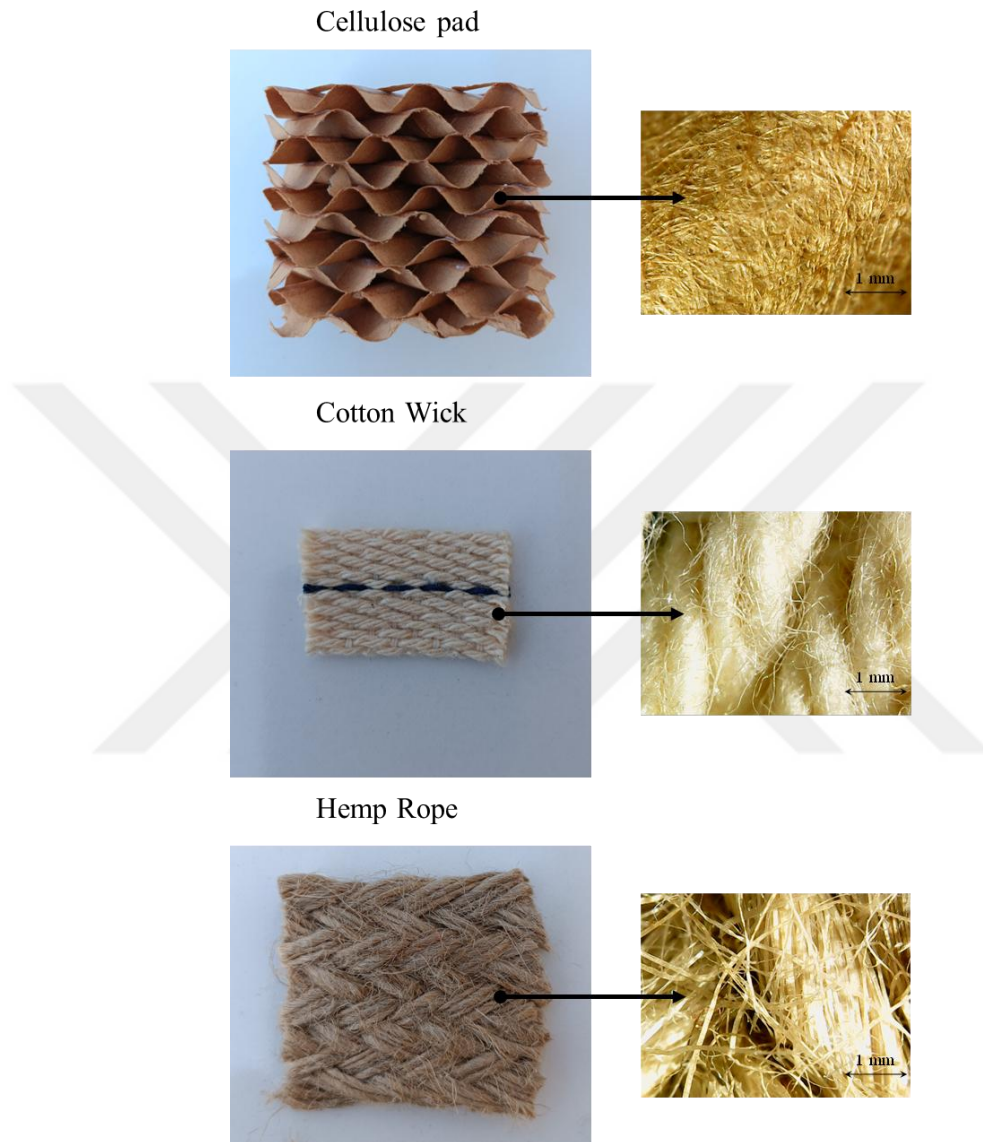
Figure 7.15. Cooling materials and their microscopic structures
