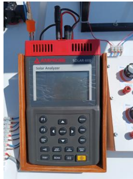
Figure 7.9. Solar power analyzer
