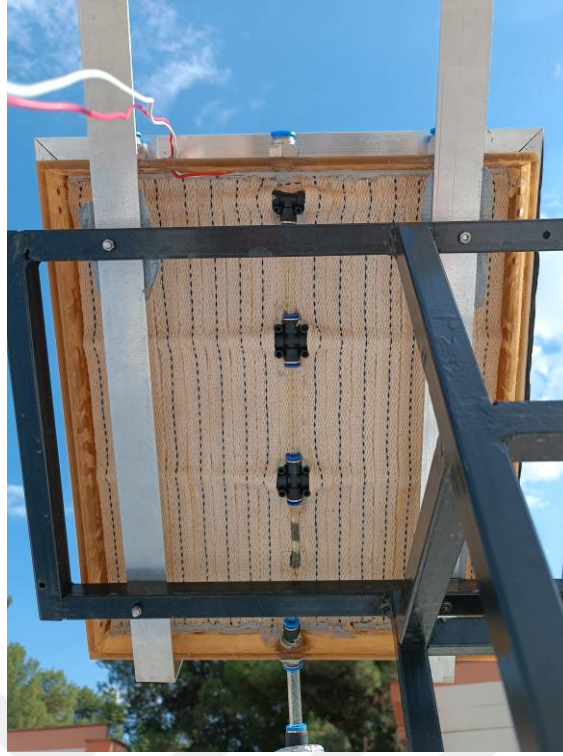
Figure 7.26. Experimental setup of the cooled panel
