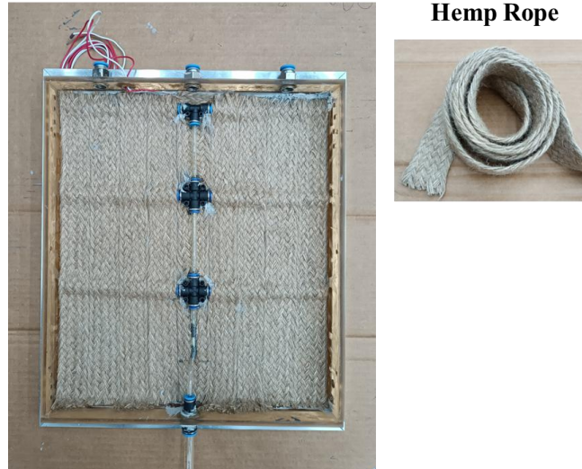
Figure 7.27. Cooled PV Panel with attached hemp rope.
